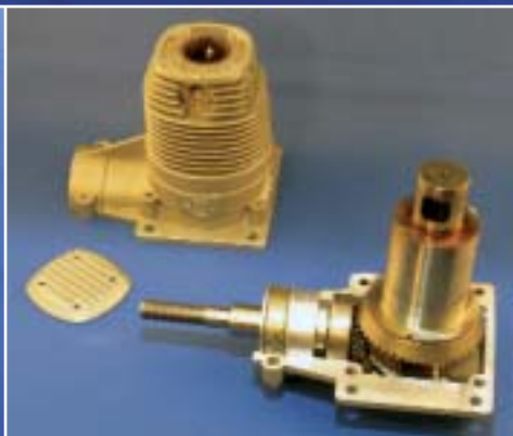
Left: With the case removed, you can clearly see the cylinder and see how it is driven off the crankshaft gear. Also note the port window.
