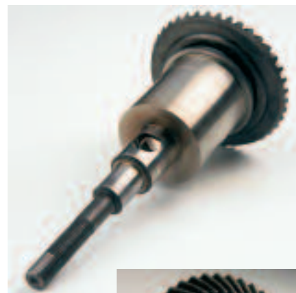
Above: here you can clearly see the rotating-sleeve/propshaft component. Note the single port cut into the large forward portion. It acts as both the intake and exhaust ports. Left: at the aft end of the sleeve is a large helical gear. It mates with the small gear that's driven by the crankshaft at the back of the engine case.
