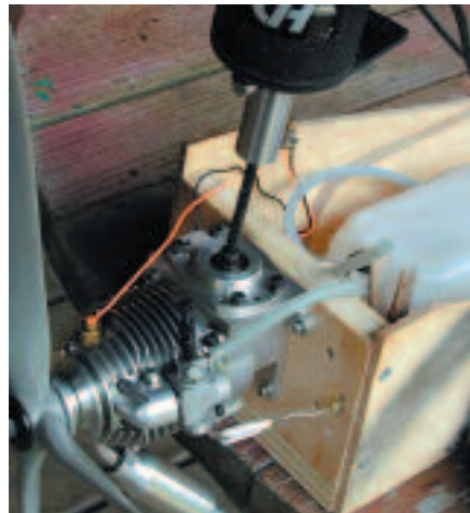
Only start the engine with the behind-the-prop-starting wand. It is both easier and safer to start the engine this way.
