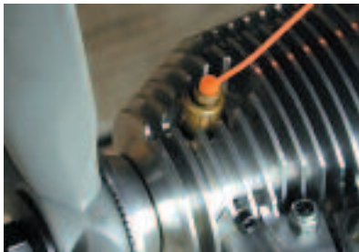
For safety, use a glow-plug extension wire and a remotely located glow-driver connector. The glow plug is extremely close to the prop, and you should not attach your Ni-Cd driver battery directly to the plug.
