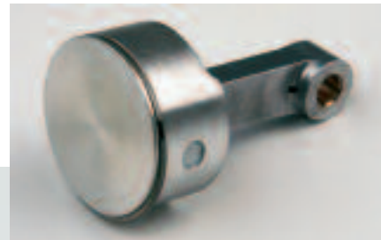
The ringed piston looks quite ordinary. Note that the oil hole drilled into the conrod's lower end faces toward the piston.
