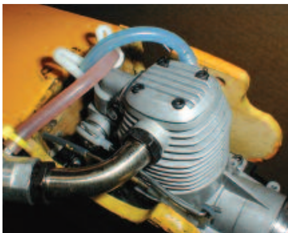
The RCV58-CD fits nicely in the test plane; the author used an articulated throttle linkage to manage the carburetor placement.
