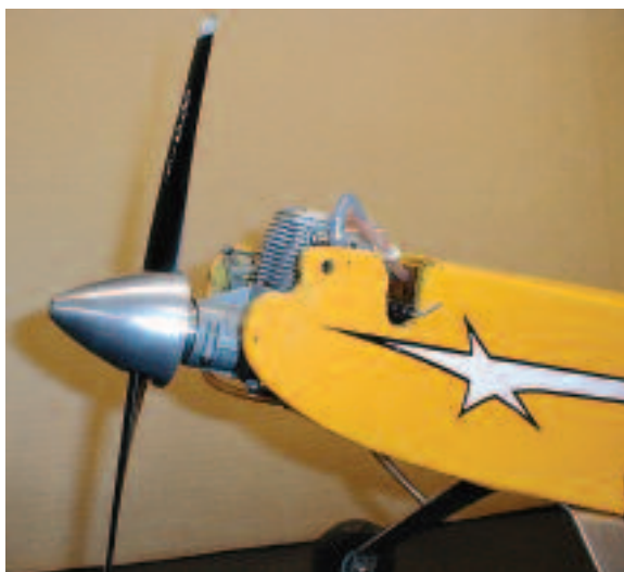
The Sig Four-Star 40 served as the test plane. It performed well with both the Master Airscrew 12x6 (shown) and the APC 11x7.
