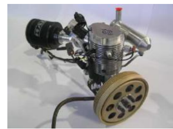
DF35 - Air cooled with Generator
